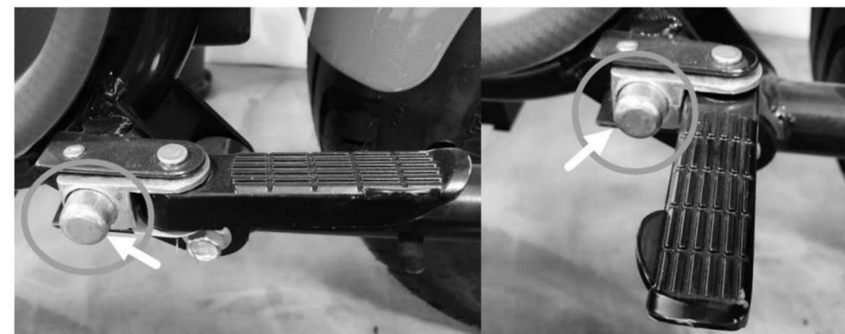
→ Passenger foot support operation: When using, hold down the arrow to open it, when it is not necessary, put it back!
